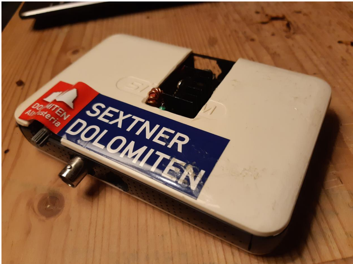
Pixie transceiver, 7023 kHz, 900 mW in a modem box.
