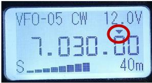
**VFO Tuning Steps:** The VFO tuning steps are set / changed by pressing down *momentarily* on the **Tune** control. Press briefly to change tuning steps. (Observe location of triangle (**carat**) above digit) The tuning steps for the VFO are (R to L) 10Hz, 100Hz, 1KHz and 100KHz.
